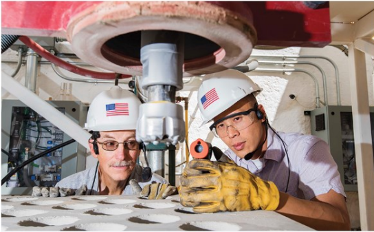
Atlas Copco has teamed up with Sandia National Laboratories to develop a DTH hammer capable of drilling geothermal boreholes in temperatures as high as 572 degrees Fahrenheit. Source: Sandia National Laboratories
